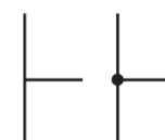
junction of conductors
